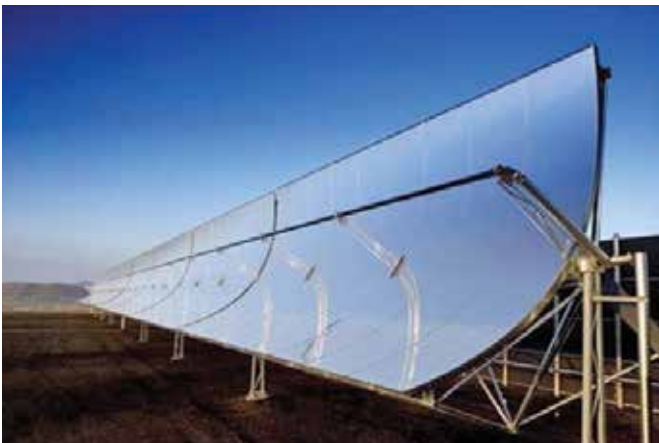
Figure 1: Parabolic trough concentrator
