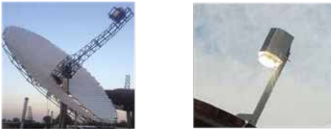
Figure 3: Paraboloid dish concentrators and receiver
