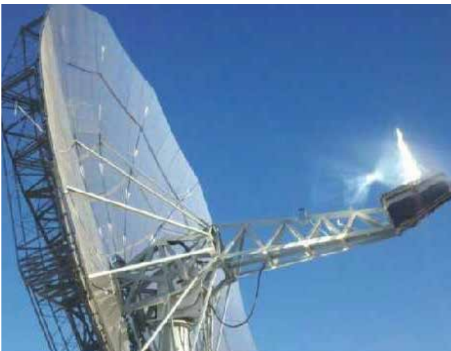
Figure 1: Solar paraboloid dish concentrator
