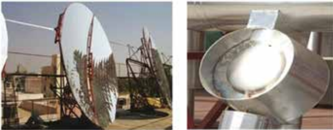
Figure 3: Reflector and receiver of Scheffler dish system
