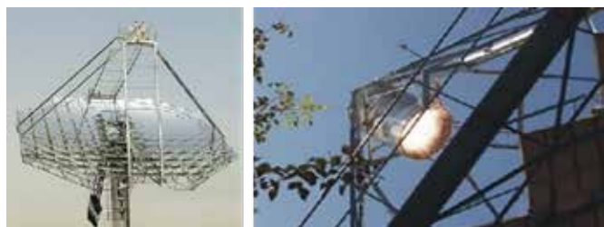
Figure 4: Collector and receiver of ARUN dish
