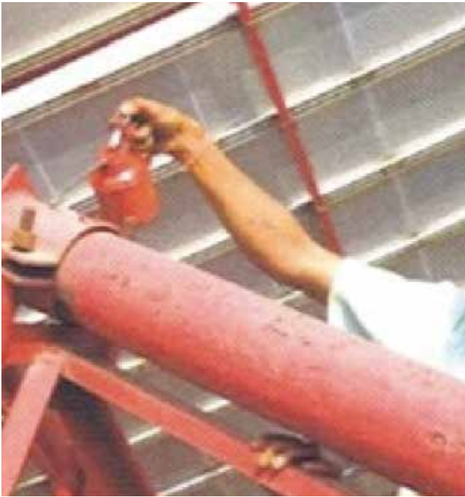
Figure 8: Greasing of moving parts
