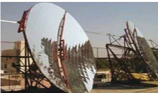
Figure 1: Fixed focus elliptical (Scheffler) dish
